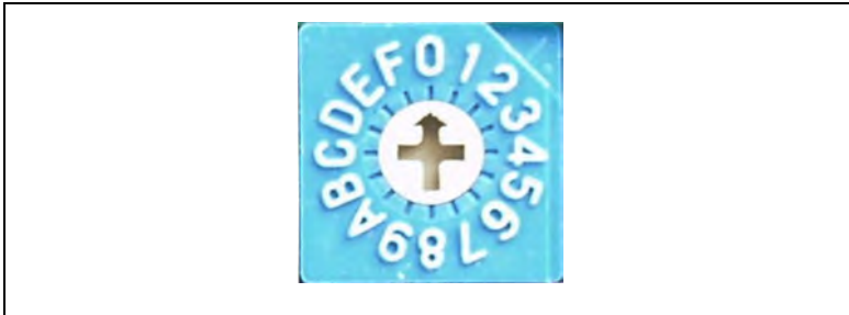
Fig. 15: 16-step rotary switch: Setting 0...F
